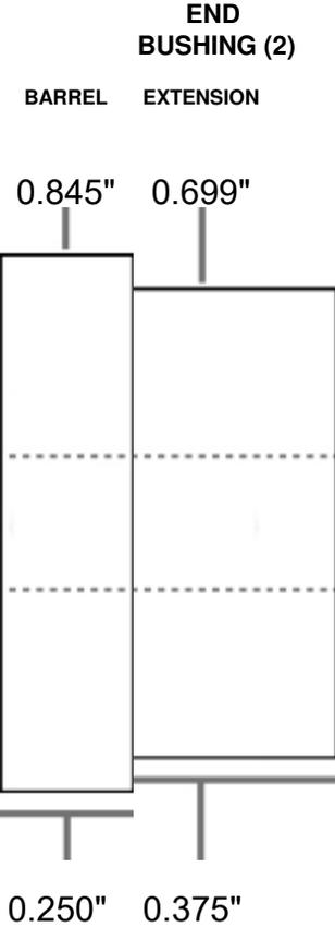
**PICTURE IS AN APPROXIMATE REPRESENTATION. NOT TO EXACT SCALE OR PROPORTION. ALL MEASUREMENTS IN INCHES. BUSHING DIAMETERS (TOP ROW) ARE OPTIMAL AND SHOULD VARY BY NO MORE THAN .002" WHEN NEW.**
